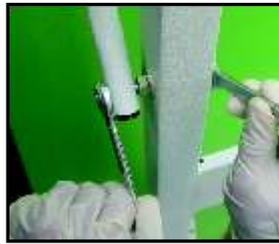
Attach long brace support P2 with outer leg P1 using nut 8mm and tighten it with the help of two spanners.
