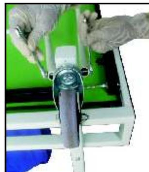
Attach long brace support P2 & small brace support P3 with wheel assembly P4 using nut and both P22 - 100x8mm and tighten it with the help of two spanners.
